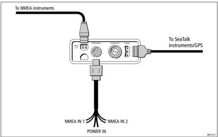
Figure 6-7: Chartplotter Display Connector Panel
